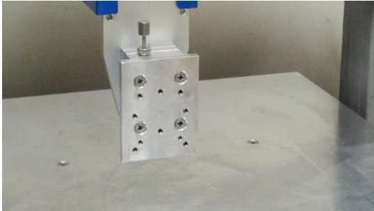
1. Move and lower head using teaching pendant.
